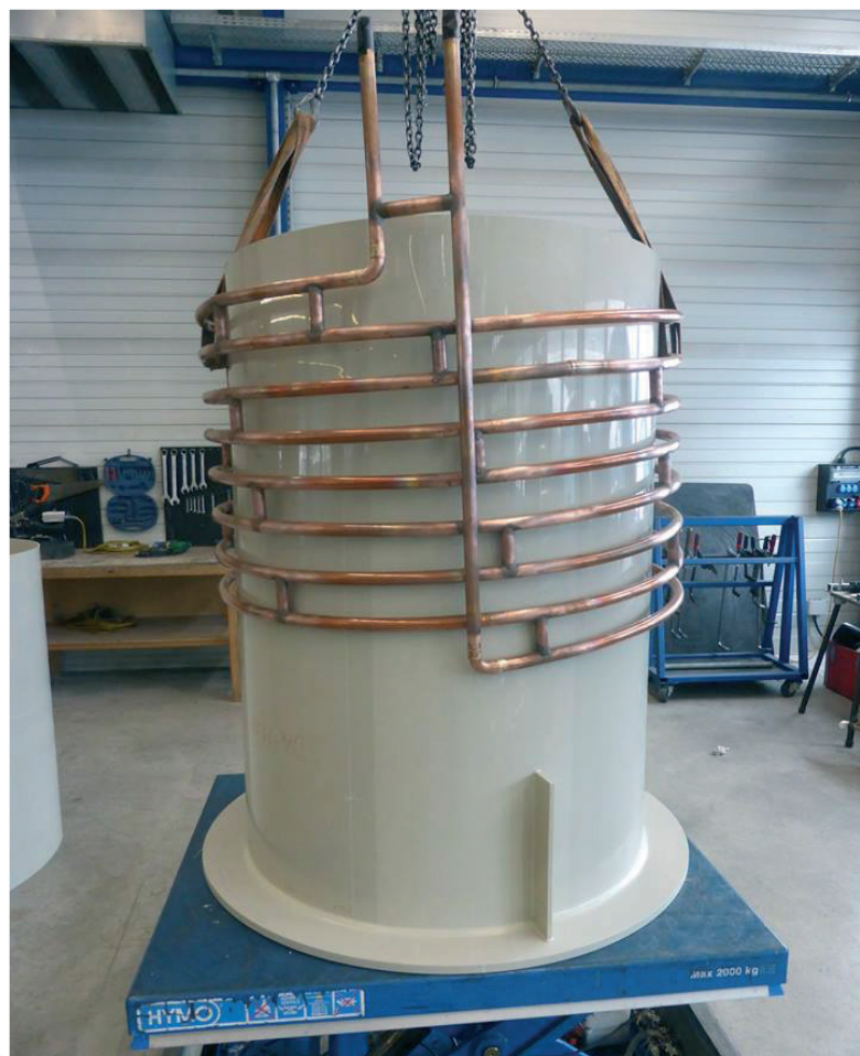
Tank for homogenisation with cooling loop
