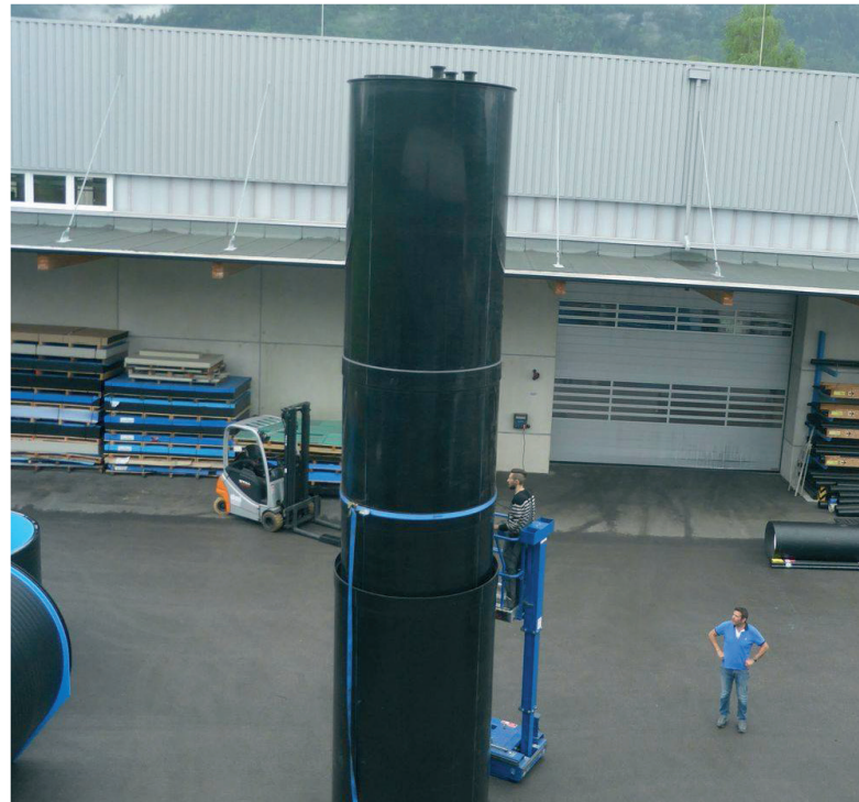
PE circular tank with collection tray to store 40% urea
