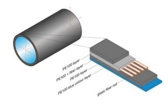
We always design a solution, in which the fibre is concentrated in just a thin layer in the middle of the PE 100 structure. This method guarantees the necessary PE thickness for a high-quality welding.
