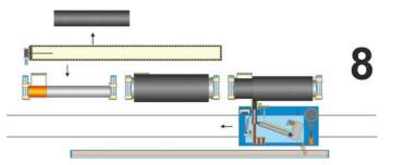
The winding of the third pipe starts, the first pipe (with the mandrel inside) already cooled down and is transported to the dismantling station
